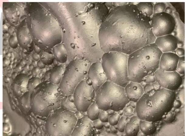
**Figure 2: Copper flotation froth**
