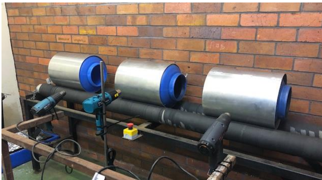
Figure 2: Aeon Heap Leach Bottle Roll Setup (ALS Burnie, Tasmania)
