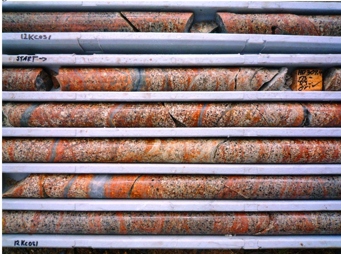
**Figure 8 Below:** Shows a D vein (In the terminology of Gustafson and Hunt) with Molybdenite and Chalcopyrite in highly altered biotite granite intrusive at 280m in KD045.
