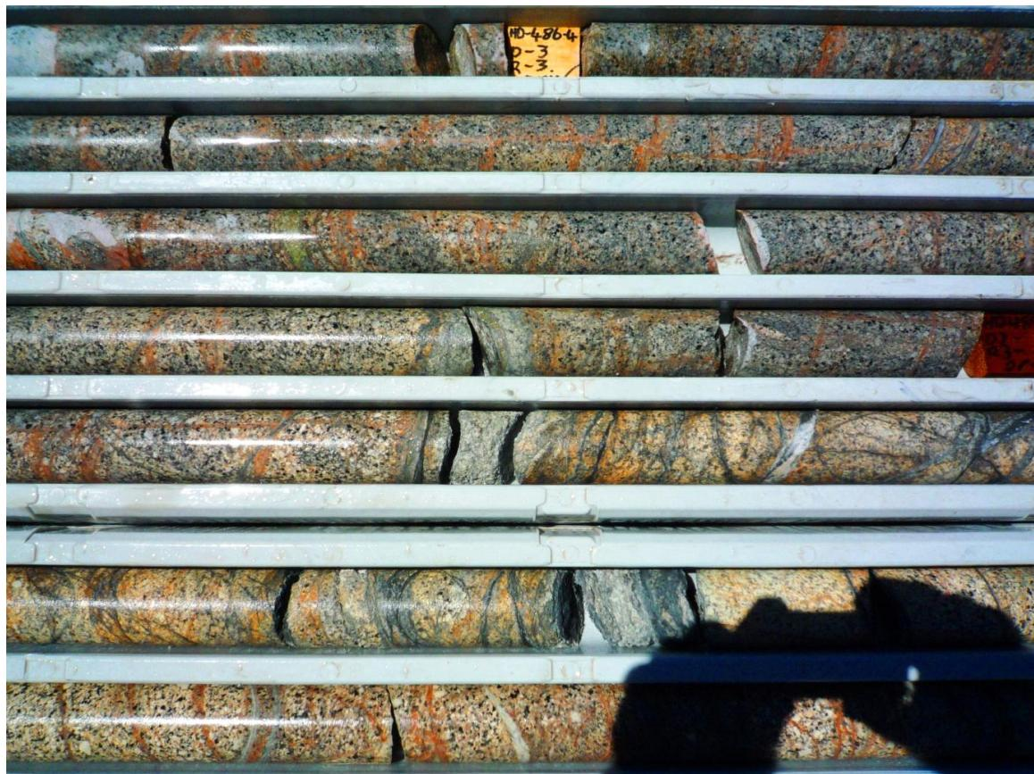
**Figure 5 Below: Stockwork with Molybdenite and Chalcopyrite in highly altered biotite granite intrusive at 402m in hole KC051. Note the intensity of veining.**
