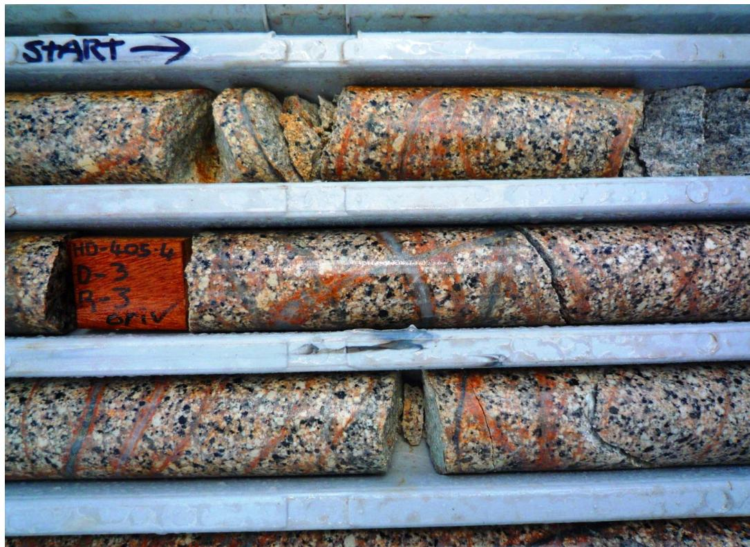
**Figure 7 Below: Stockwork with Molybdenite and Chalcopyrite in highly altered biotite granite intrusive at 309m in hole KD051.**
