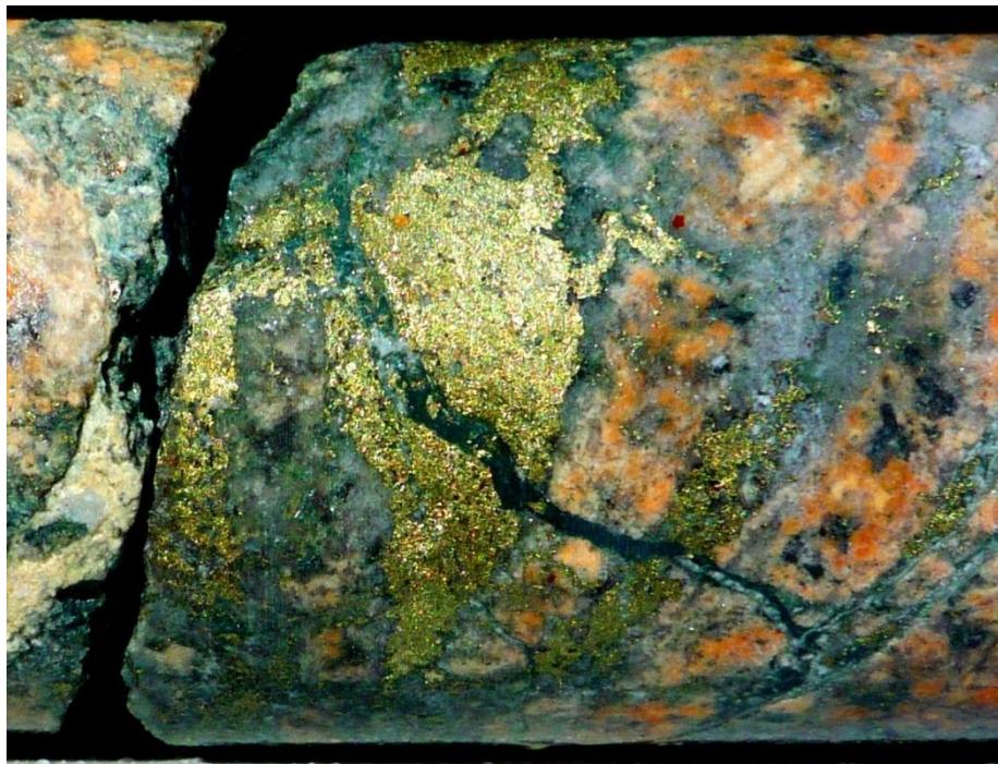
**Figure 4:** Disseminated chalcopyrite in biotite monzonite intrusive at 259m in Hole 55.
