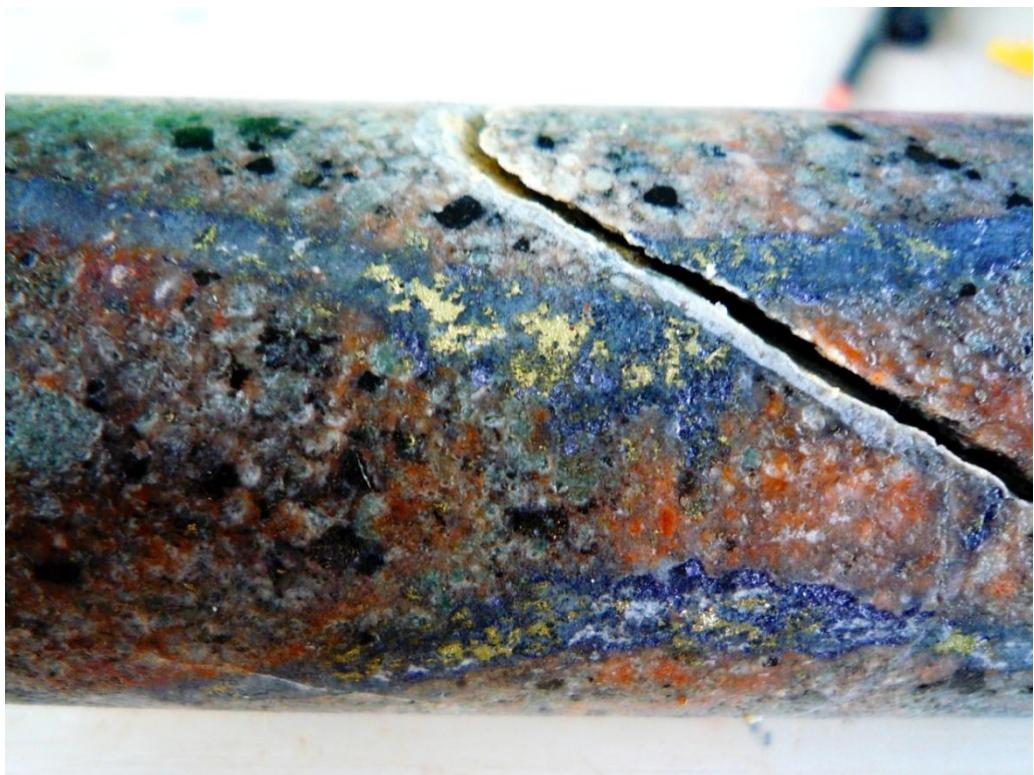
**Figure 6:** Molybdenite and chalcopyrite in B vein at 468m in Hole 55. Sample 467m to 468m assayed 0.62% CuEq<sup>1</sup> consisting of: 0.45% Cu, 323ppm Mo & 2.6g/t Ag
