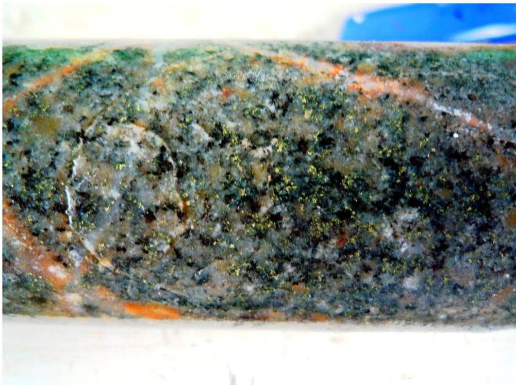
**Figure 5:** Close up view of the molybdenite and chalcopyrite in biotite monzonite intrusive at 288m in Hole 55. Sample 287m to 288m assayed 0.92% CuEq<sup>1</sup> consisting of: 0.44% Cu, 0.11% Mo & 3.3g/t Ag.
