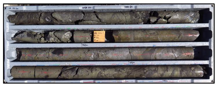
Figure 2 Shows Tray 84 from hole WFDH347 at 401.1m to 404.2m. Zone of massive, semi-massive pyrite, chalcopyrite and sphalerite.
