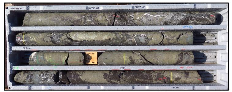
Figure 1 Shows Tray 106 from hole WFDH346 at 419.1m to 422.1m. Massive to semi-massive pyrite and chalcopyrite.
