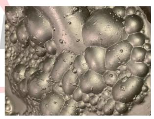
Figure 2: Copper flotation froth
