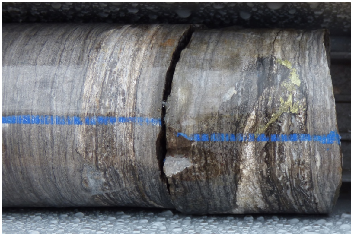
Figure 3. Chalcopyrite vein within a carbon rich section of the Walford Dolomite (WFDH483, 195.7m)
