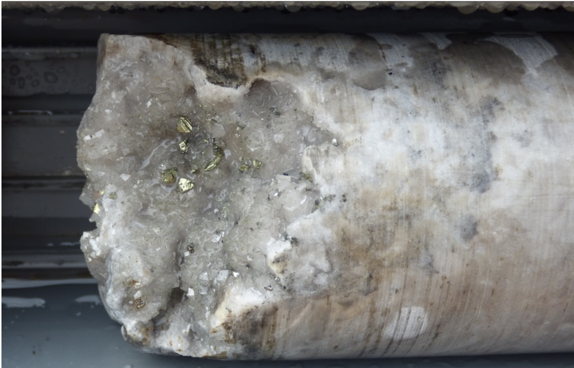
Figure 2. Euhedral Chalcopyrite crystals with Quartz Carbonate veining within the Walford Dolomite (WFDH483, 190.4m)
