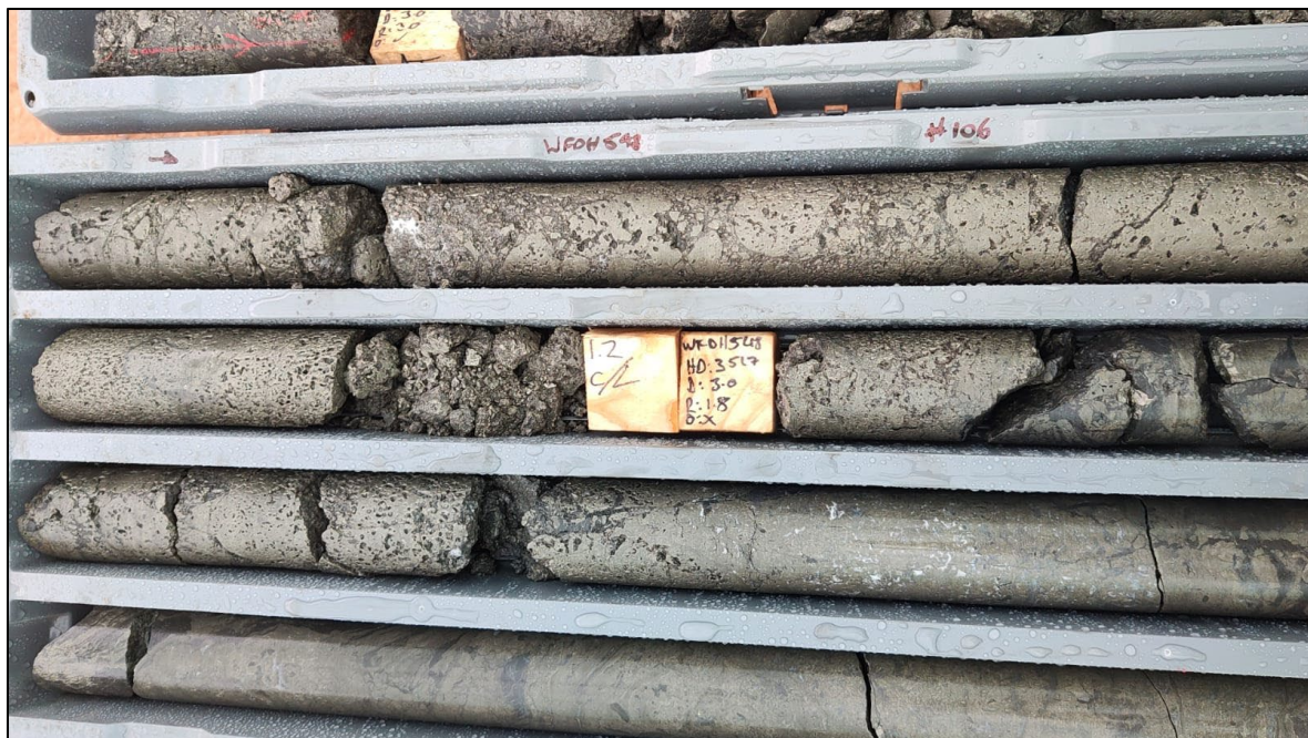
Figure 2: Drill core from WFDH548 showing massive to breccia replacement sulphide mineralisation at Amy West
